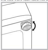
1. Install the washing machine on a flat sturdy floor, without resting it up against walls, cabinets or anything else. 2. If the floor is not perfectly level, compensate for any unevenness by tightening or loosening the adjustable front feet (see figure); the angle of inclination, measured according to the worktop, must not exceed 2°.
